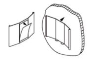
Wall-mounting with double-sided adhesive for codes: 5129-BA
