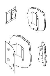
Wall-mounting with a steel plate with a double-sided adhesive for codes: 5130-BA, 5131-BA, 5134-BA.
